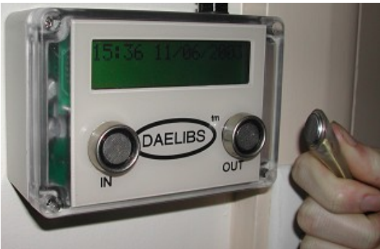
Clock connected into Local Area Network
