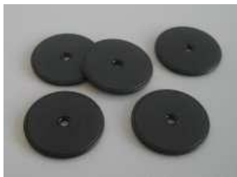
RFID Proximity Tags. Black or beige Tags 20mm and 30mm Plastic Disk. 125KHz RFID chip encapsulated in a Plastic Disk. The plastic disks can be embedded in wood or plastic. Ideal for tropical climate locations. Proximity read range of 2cm.
