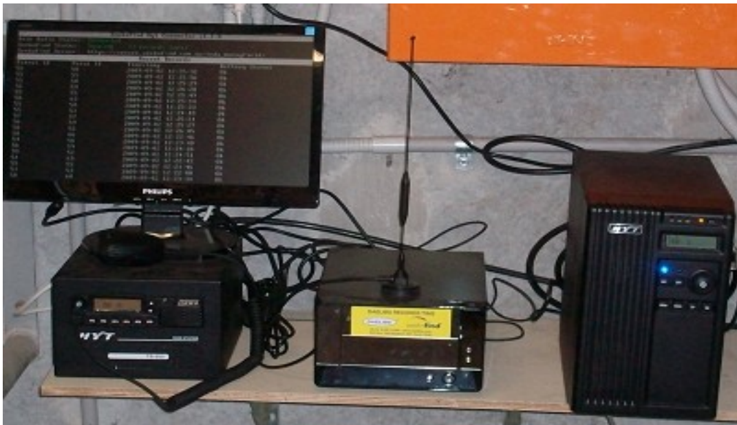
The HYT Data Reception Base Radio and SeeknFind Raw Data Display Monitor.
